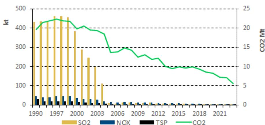
**Figure 3.3.5** Measured emissions from large electricity plants (1990-2023) Source: Data of the Hungarian Electricity System, 2023
