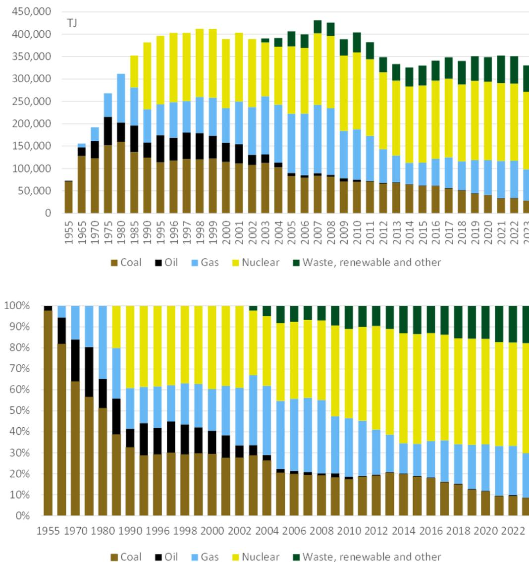
**Figure 3.3.3** Energy consumption of power plants (above) and the share of different energy sources in power production (1955-2023)<sup>1</sup>
